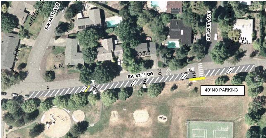
Figure 9. Reverse Angle Parking on SW 47 th Drive
