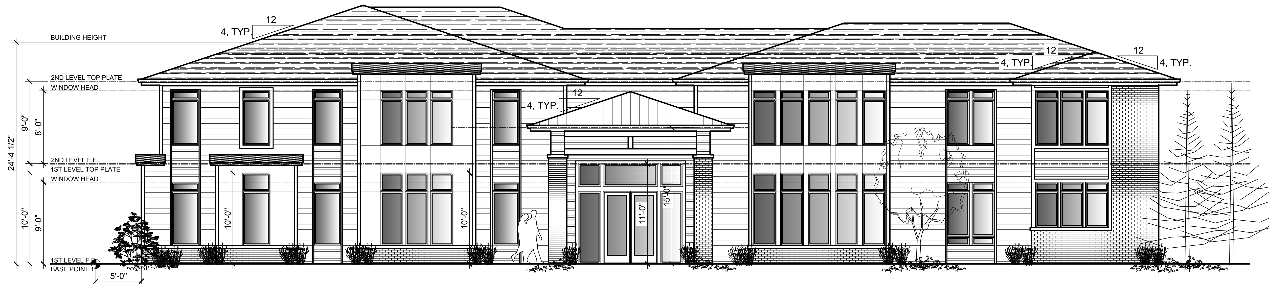
A REAR ELEVATION (MAIN ENTRY) A2.0 SCALE: 3/16" = 1'-0"
